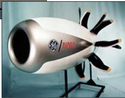
Right: NASA / GE Unducted Fan Engine
