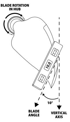
**d.** Torque the 5/16" Blade Clamping Bolts to **16 ft-lbs**. before operating propeller.
