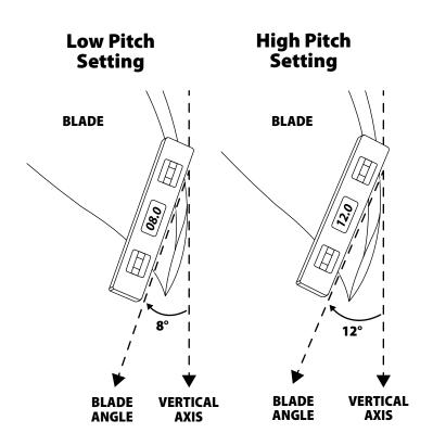
**WARNING:** Never use a mallet or other object to tap the blade during pitch setting.
