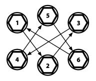
c. Torque 1/2" Mounting Bolts to40 ft-lbs.
