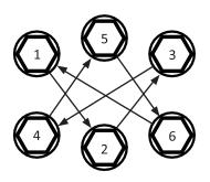
**c.** Torque 1/2" Mounting Bolts to **40 ft-lbs**.
