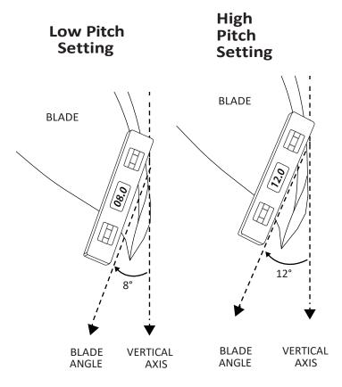
**WARNING**: Never use a mallet or other object to tap the blade during pitch setting
