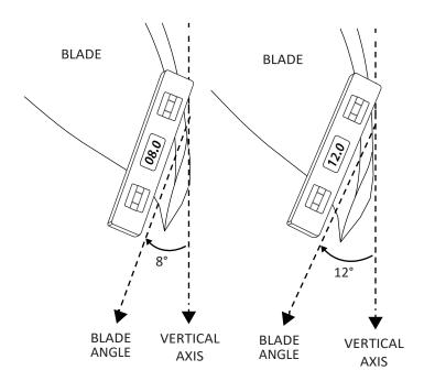
warning: Never use a mallet or other object to tap the blade during pitch setting.
