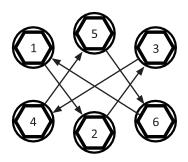
**c.** Torque 5/16" or 8mm Mounting Bolts to **16 ft-lbs**.
