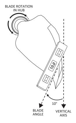
**d.** Torque the 5/16" Blade Clamping Bolts to **16 ft-lbs**. before operating propeller.
