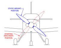
**Propeller Clocking:** The historical installation position of a two blade propeller is to place the upper blade in the 10 o'clock position as shown above.
