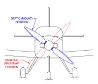
**Propeller Clocking:** The historical installation position of a two blade propeller is to place the upper blade in the 10 o'clock position as shown above.
