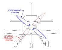
**Propeller Clocking:** The historical installation position of a two blade propeller is to place the upper blade in the 10 o'clock position as shown above.
