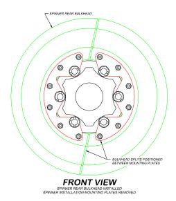
Install the spinner dome onto the propeller hub and rear bulkhead. The spinner and spinner rear bulkhead have been number coordinated to match the blade cutout openings.
