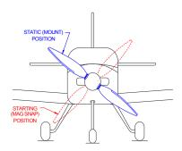
**Propeller Clocking:** The historical installation position of a two blade propeller is to place the upper blade in the approximate 10 o'clock position as shown above.
