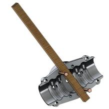
↑ To torque bolts, follow tightening pattern below and tighten in the following increments: 50%, 75%, then Full Torque.
