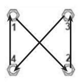
**Broom Trick:** Temporarily install forward hub's mounting bolts and place a broom stick between them while you torque desired mounting bolts.
